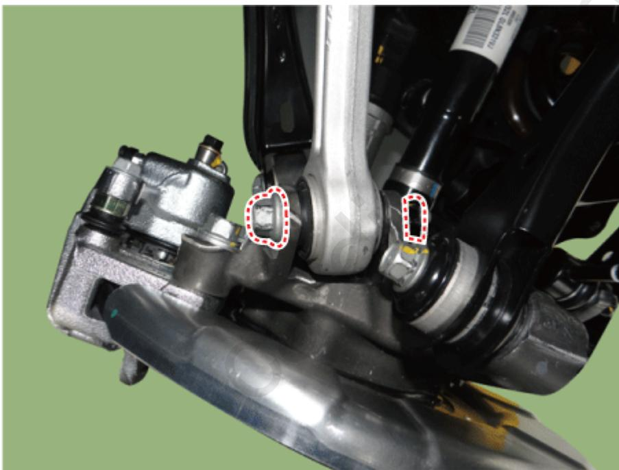
11. Loosen the rear upper arm rear bolt & nut (A) and then separate the rear upper arm rear.
